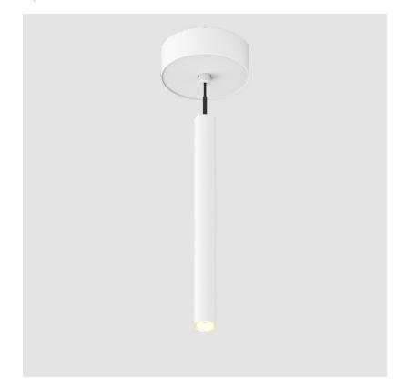
Fixture Material: Aluminum Cable Details: 2000mm or 4000mm Black Cable **ELECTRICAL** Lamp Type: LED (Zhaga Standard) Input Wattage (W): 6.6 Total Output Wattage (W): 6 Dimming: Tri-Mode (Non-Dimming and Phase Dimming (120Vac only) and 0-10V Dimming) Driver Included: Yes Driver Location: External Driver Type: Constant Current - Universal Driver Class: Class 2 Housing: ENCP3 w/quick connect Input Voltage (V): 120 - 277 Constant Current (MA): 500 LED
