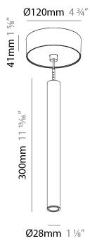
Color Temperature (°K): 2700 / 3000 / 4000 Max. Delivered Lumen (lm): 330 / 350 / 370 CRI: >90 CRI Efficiency (%): 86
